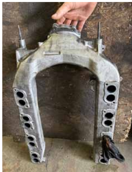
Inlet manifold showing rag blocking #6 cylinder ports
